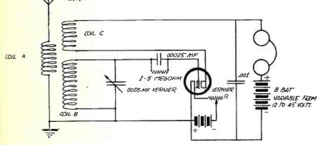
Figure 2. The wiring diagram of the Simplifigon receiver. This type of set is a very desirable one to the bug who is interested in speedy tuning, inasmuch as it has only two major controls and two minor ones. The 23 plate condenser and the tickler are about the only ones that need adjustment after the set has been adjusted in the filament and antenna circuits. Due to the fact that the apparatus is of low loss design and of small quantity the receiver will cover unusual distances.
