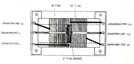
the same frequency Figure 6. This illustrates the method of making the connections for the inside and when it reaches the outside coils of the oscillator unit. The center lug is used for the inside (L5) coil, and r a d i o frequency the two outside lugs form the terminals for coils L3 and 4 respectively.
