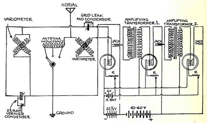
Figure 4. The Kopprasch circuit in connection with two stages of audio frequency amplification. A receiver of this type will bring in distant stations with considerable volume on the louds peaker. Amplifying transformer No. 1 should have a ratio of about 3 1-2 or 4 to 1 while the second should have a ratio of not greater than 6:1.
