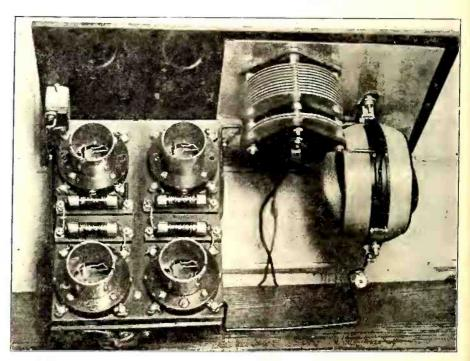
The above photographs picture a method used by a radio fan to eliminate controls for the filaments of the tubes. The cartridge types of resistance are of the proper value to be used instead of rheostats, thereby making the use of four extra controls unnecessary. The circuit is the conventional single circuit using a variocoupler as tuner. The panel view shows how simple the control of this set is. (Kadel & Herbert Photo.)
